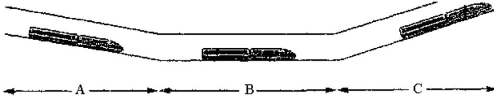
For safety reasons, the train must maintain a steady speed through the tunnel. Even though the speed remains steady, the driving force from the motors varies.
